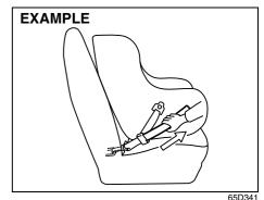
4) Return the seatback to the normal, upright position. Tighten the lower straps as described in the child restraint owner's manual. Attach the top tether strap, if applicable.
